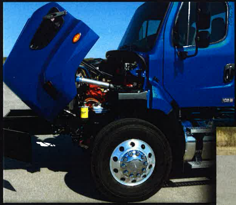
Tilt hood with radiator-mounted stationary grille for easy engine access.
